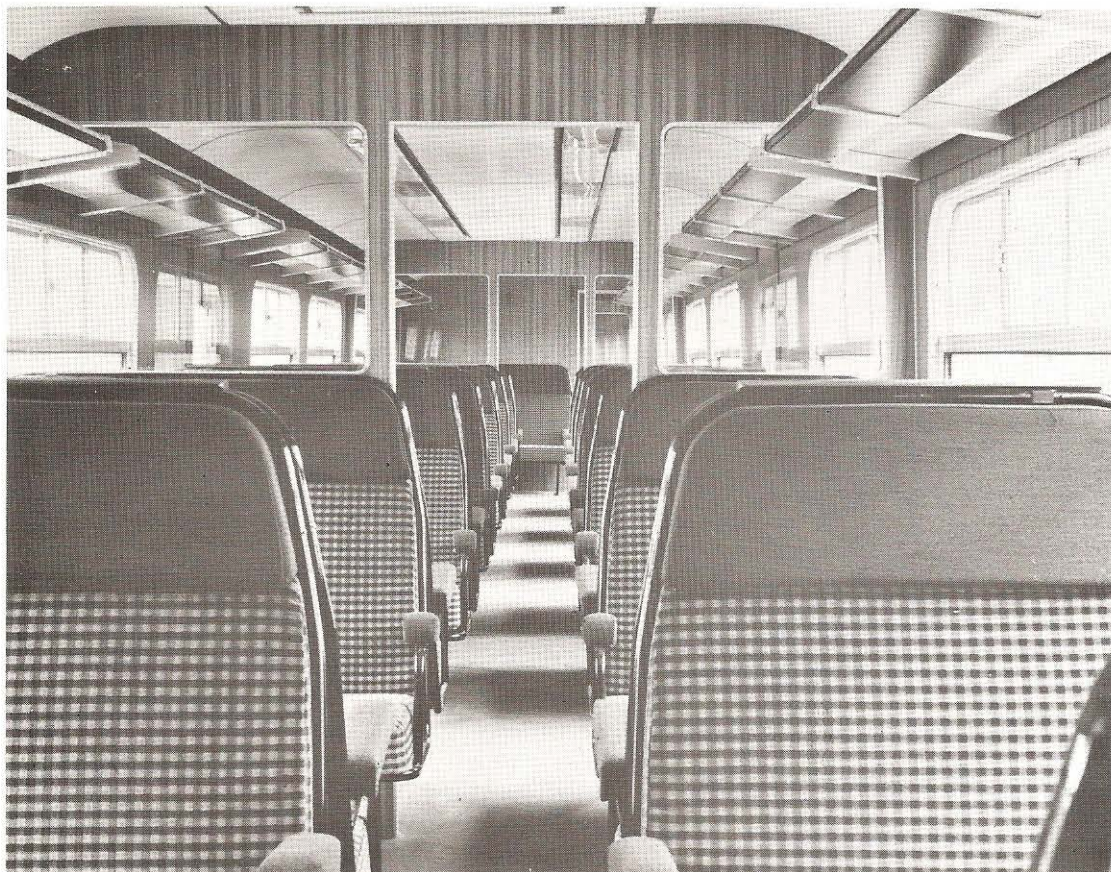
Interior of passenger saloon. All are arranged with three- and two-aside seating
