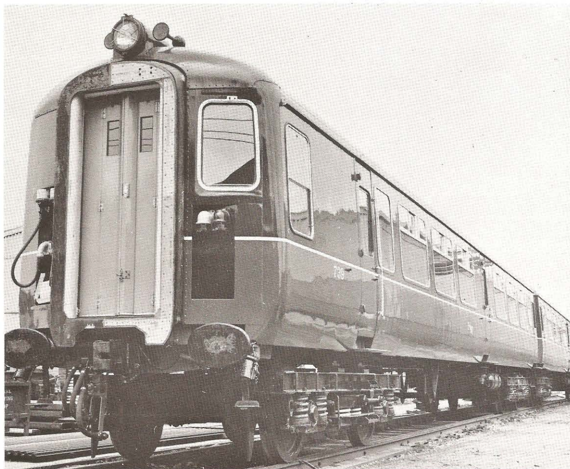
General view of Northern Ireland Railways diesel-electric mainline multiple-unit designed and built by BREL for two-three-car formation photographed at its York works
